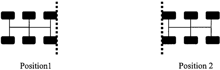
FIGURE 9: Position of wheels across the joint as test vehicle traverses the joint
