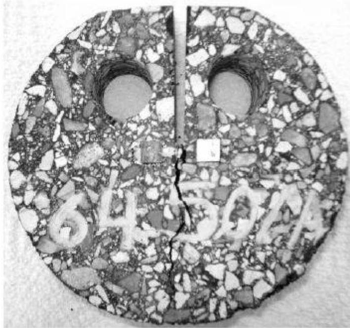
Figure 3-3. DCT Test Specimen after Test
