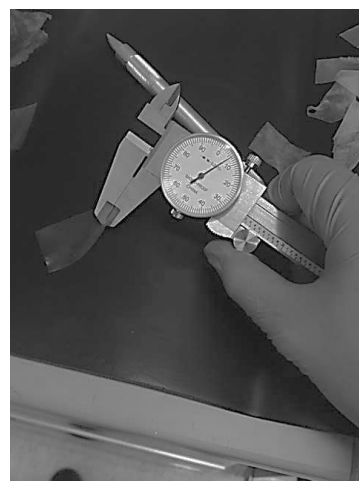
Figure 7. How to use the calipers to determine thickness
