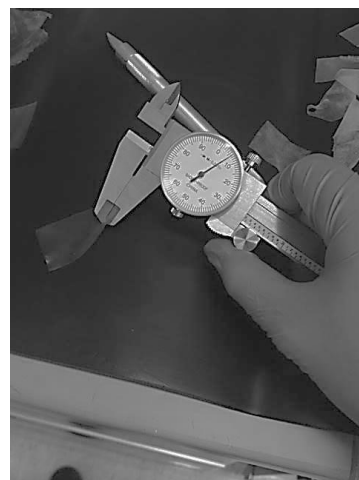
Figure 6. How to use the calipers to determine thickness
