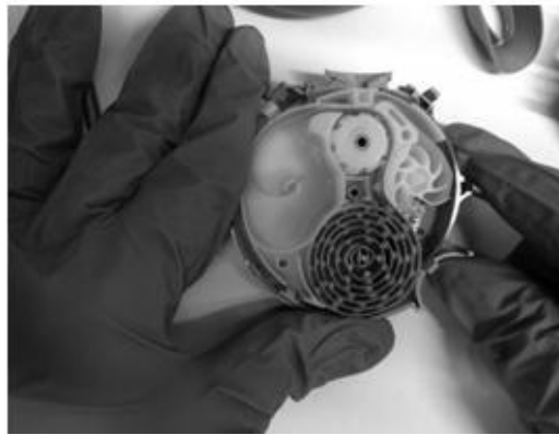
Figure 5. The inner mechanisms of an ADVAIR Diskus®.
