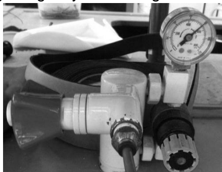
Figures 3 and 4. From left to right; the inlet air valve and the flow meter used in the fluidized bed setup.
