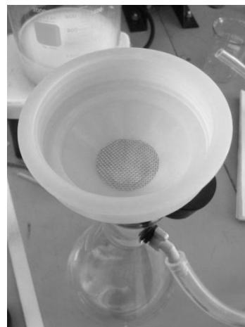
Figure 3. Funnel and screen setup for pouring into flask.
