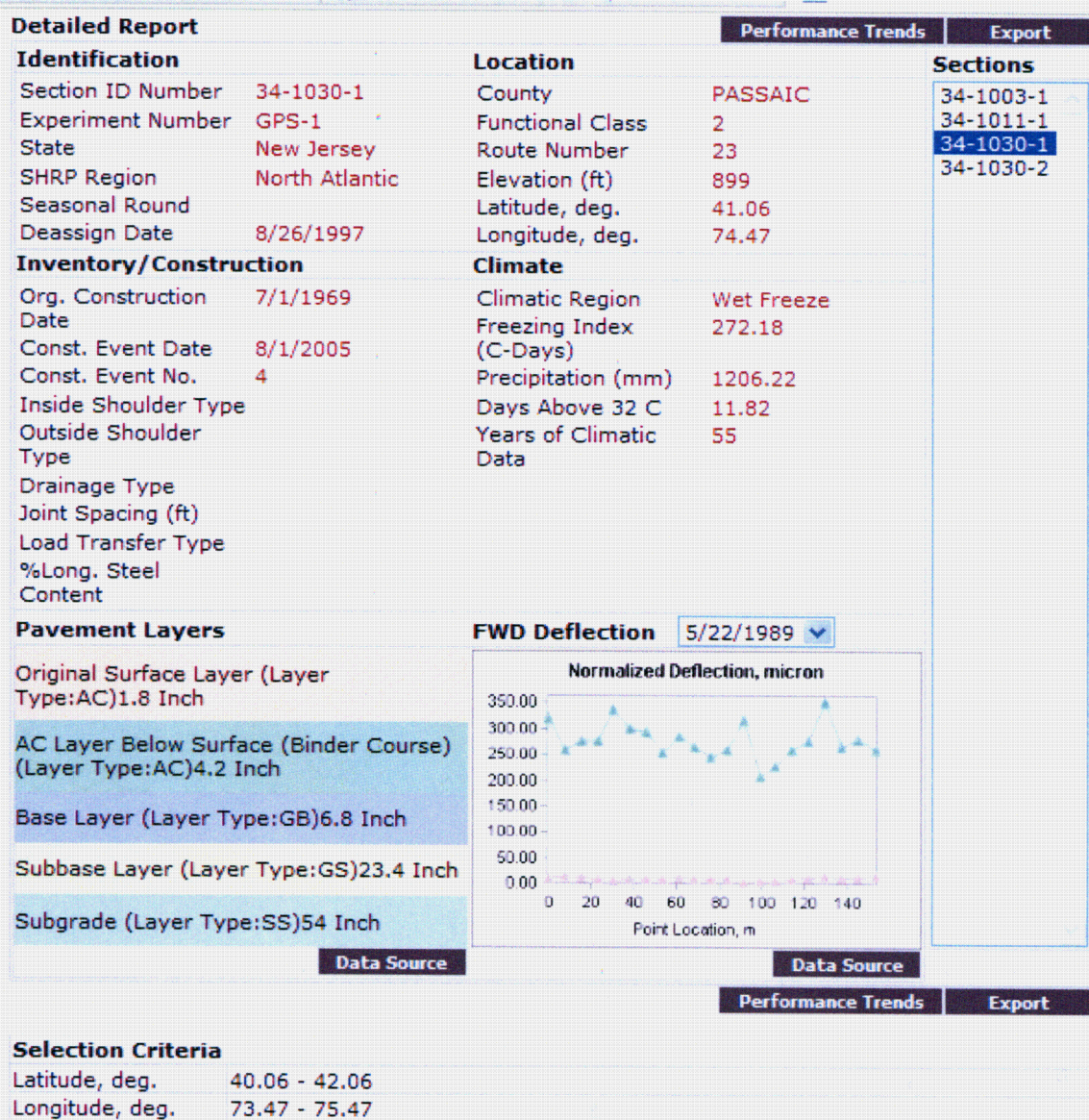
Figure 3.1 Information of Layers and Thickness for LTPP section 1030 (LTPP, 2008).
