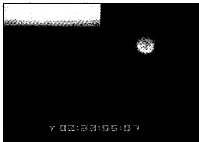
Figure 3.18: OH* emission at ignition (methanol, 1.6358 mm, 930 °C).
