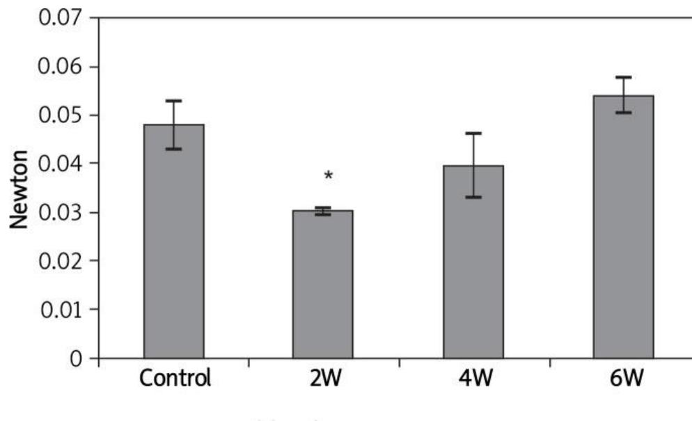
*Figure 19.* Biomechanical testing via three-point bending on SCI rats two, four and six weeks post injury versus the noninjured control group [45].
