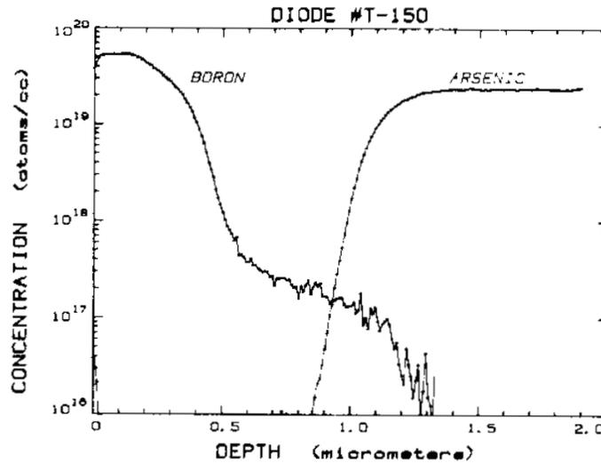
**Fig. 12**—SIMS depth profiles of epi-grown p and ion-implanted p<sup>+</sup> on n<sup>+</sup> arsenic-doped substrate.
