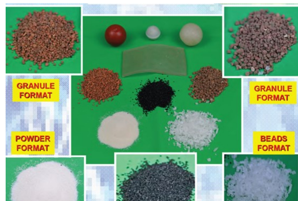
Microencapsulated phase change materials
