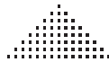
Figure 2.6: An array of bits representing the pixels making up an image of a triangle, and the image with each pixel shown as a black dot
