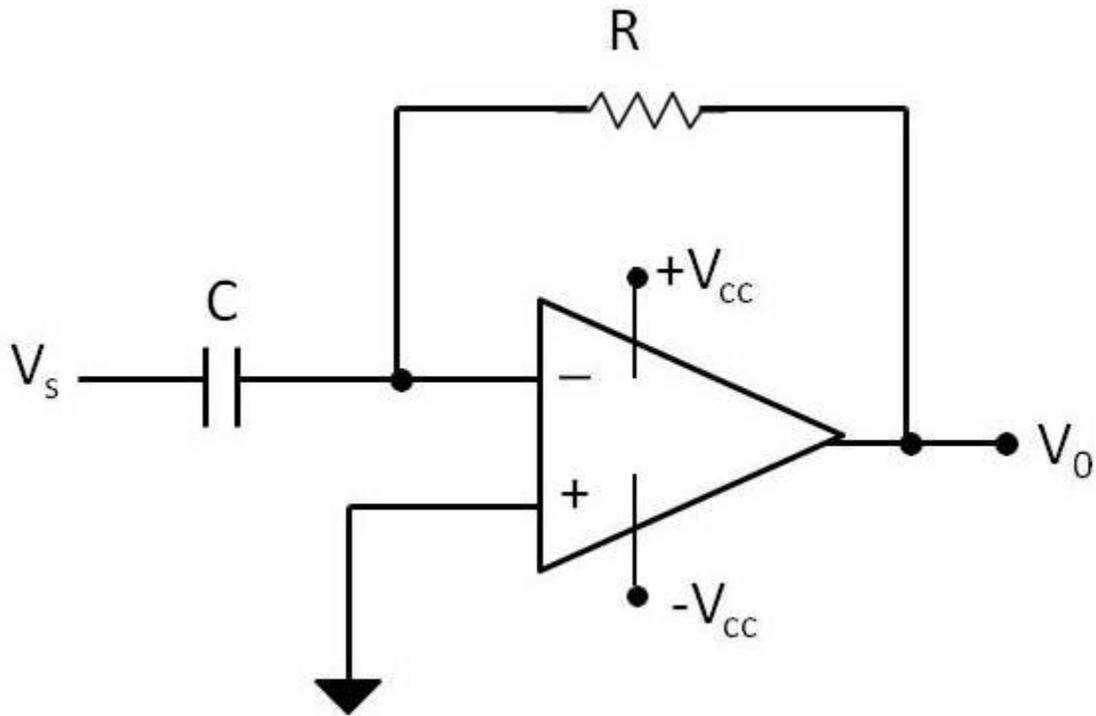
**Figure 3 – Differentiator Circuit**
