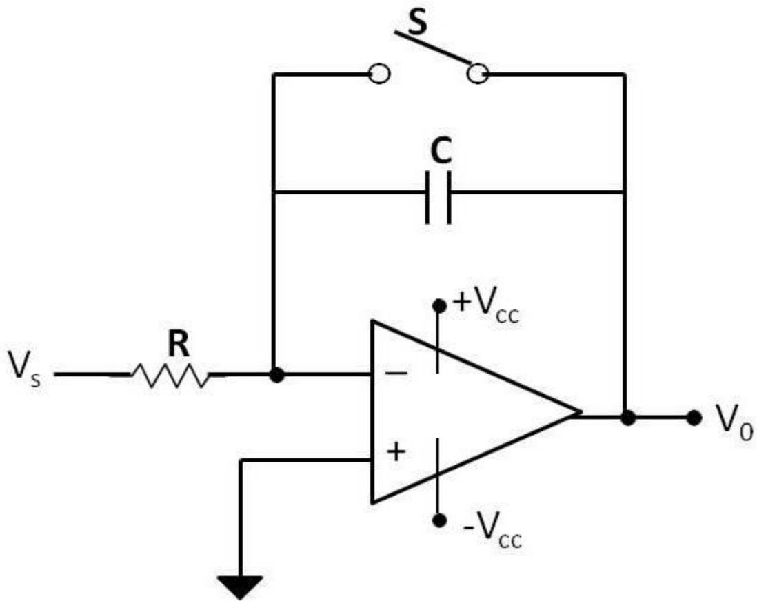
Figure 4 – Integrator Circuit
