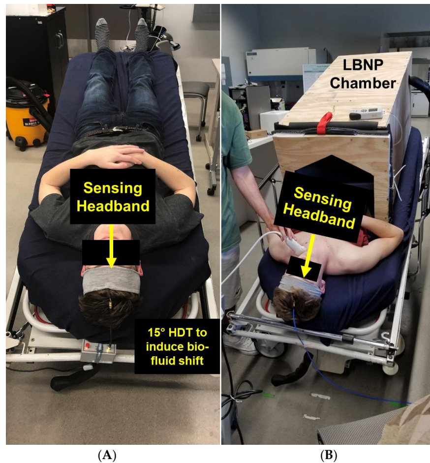
Figure 2. EM skin patch sensor embedded in wearable headband to detect induced bio-fluid shift in (A) 15° head down tilt and (B) during administration of lower body negative pressure (LBNP).
