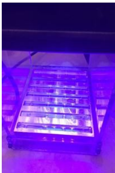
Figure 4. The mold and UV lamp apparatus used to cure resin without the use of SLA.
