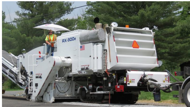
Figure 2. CIR Milling Process (Roadtec, 2019)
