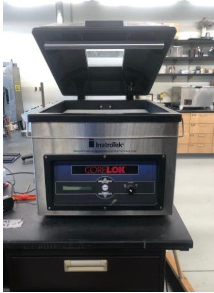
Figure 10. CoreLok Device Used to Determine Volumetric of CIR mixtures
