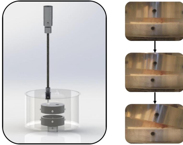
*Figure 32.* Custom-made mechanical fixtures designed to induce bending of the IVD specimen. The vertical rod is offset 25.4 mm from the center of the stainless-steel cup and affixed to a hinge allowing for rotational movement.
