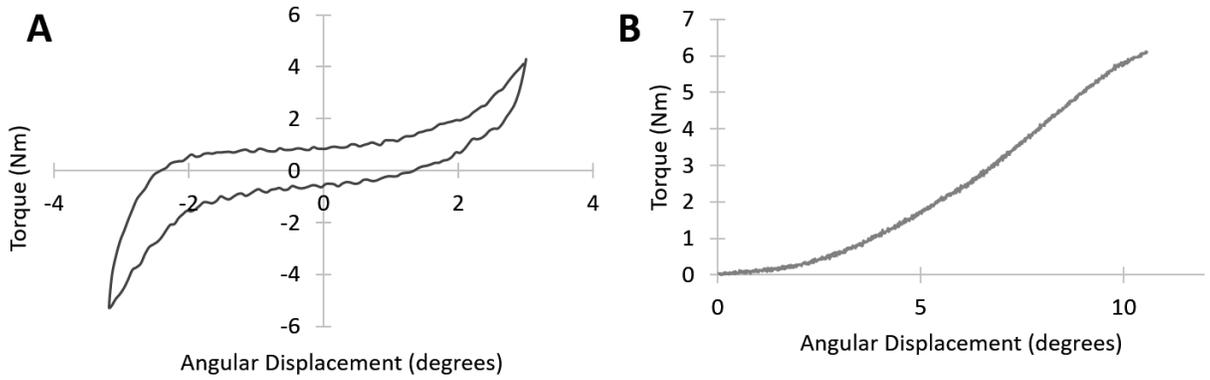
*Figure 33.* IVD specimens were punctured, denucleated, injected with composite and bent to observe potential risks for implant extrusion. (A) Representative bilateral bending hysteresis curve followed by a (B) unilateral bending expulsion test until the maximum angle of rotation was reached.
