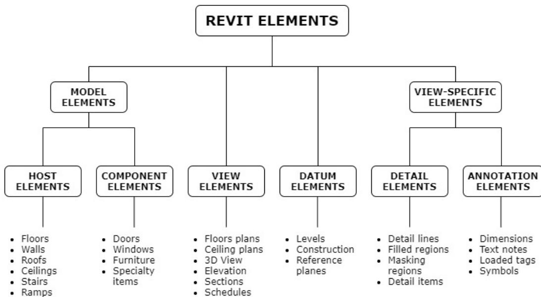
Figure 3. Hierarchy of Revit elements from Autodesk [15].
