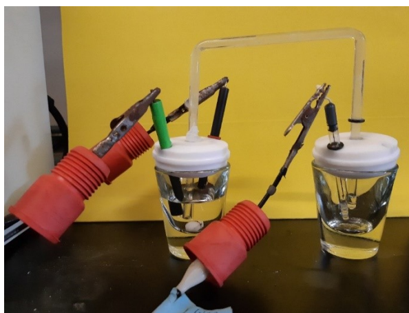
Figure 3. Carbon dioxide electrochemical conversion set-up
