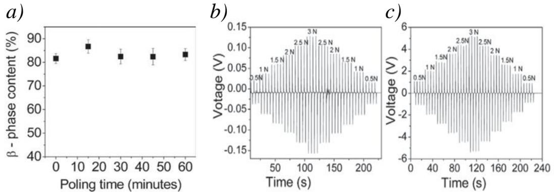
Figure 12. a) Impact of poling time on the  $\beta$ -phase content of a PVDF sample ( $T=80^{\circ}\text{C}$ ). b) Voltage output measurement of an unpoled PVDF sample and c) poled PVDF sample at  $80^{\circ}\text{C}$  for 45 min [75].
