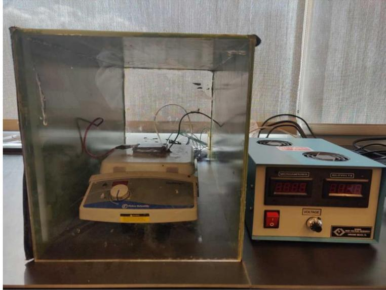
*Figure 32.* The poling setup used for the experiments.
