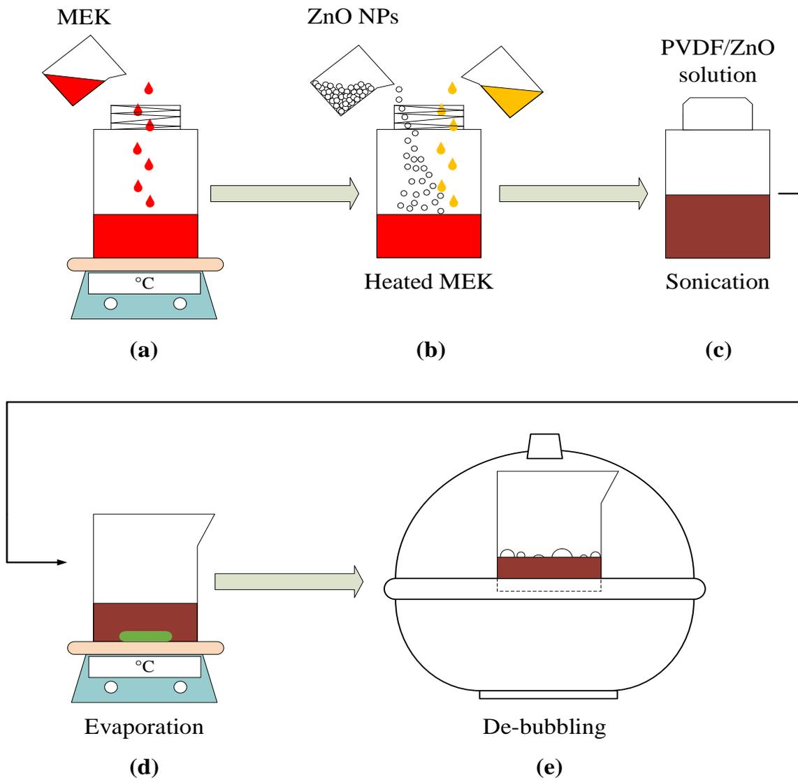
*Figure 21.* Preparation of PVDF/ZnO solution. a) MEK is poured in a 20 mL glass vial and heated up. b) ZnO NPs and PVDF solution are mixed in the glass vial. c) The glass vial is placed in sonication machine. d) PVDF/ZnO solution is poured in a beaker and placed on a hot plate for evaporation process. e) A vacuum desiccator is used for the de-bubbling process.
