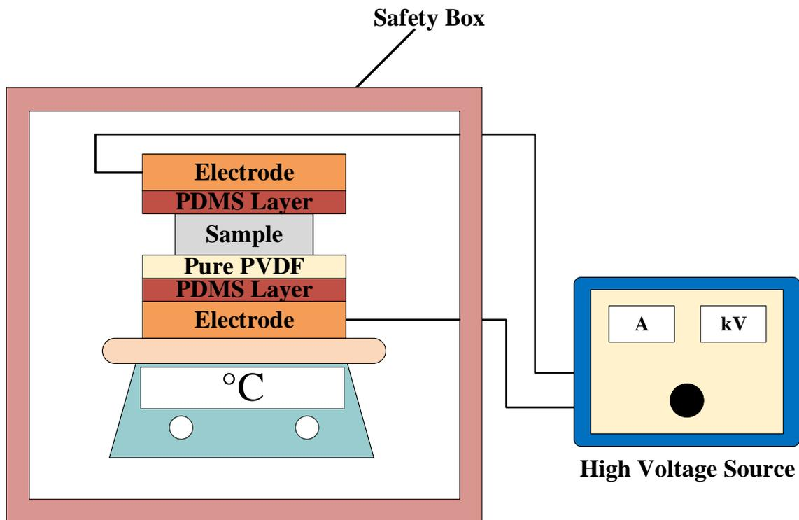
Figure 31. Schematic of the electrode poling setup.
