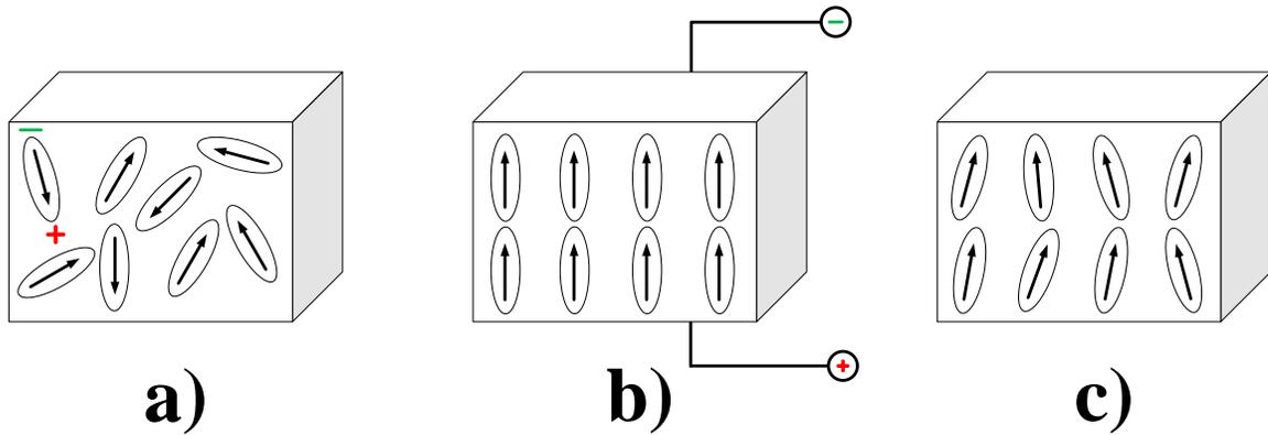
*Figure 30.* The electrode poling process to align dipoles in a material. a) Randomly oriented polar axis of domains prior to polarization. b) Reorientation of dipoles when a high electric field is applied. c) Remainder polarization after the poling treatment.
