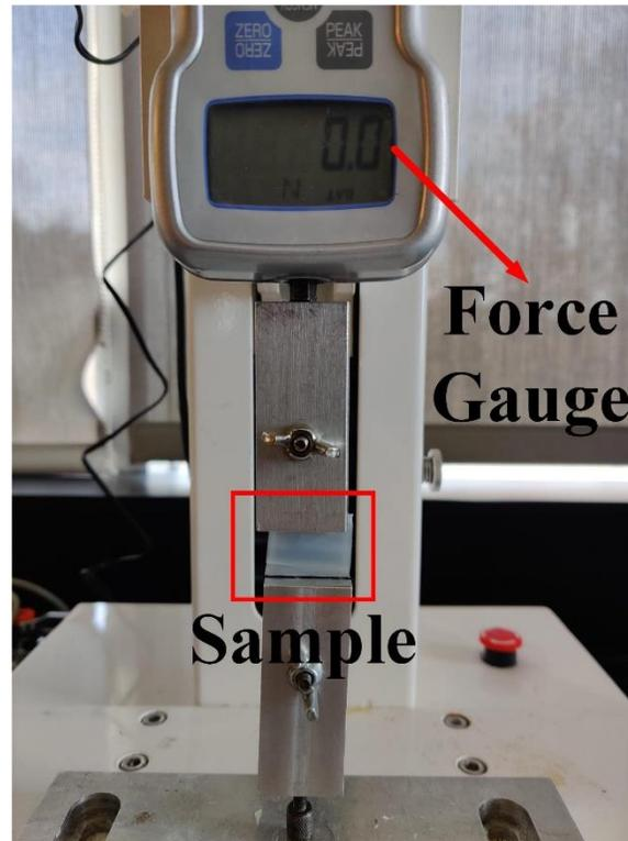
Figure 27. A mounted sample on the tensile tester.
