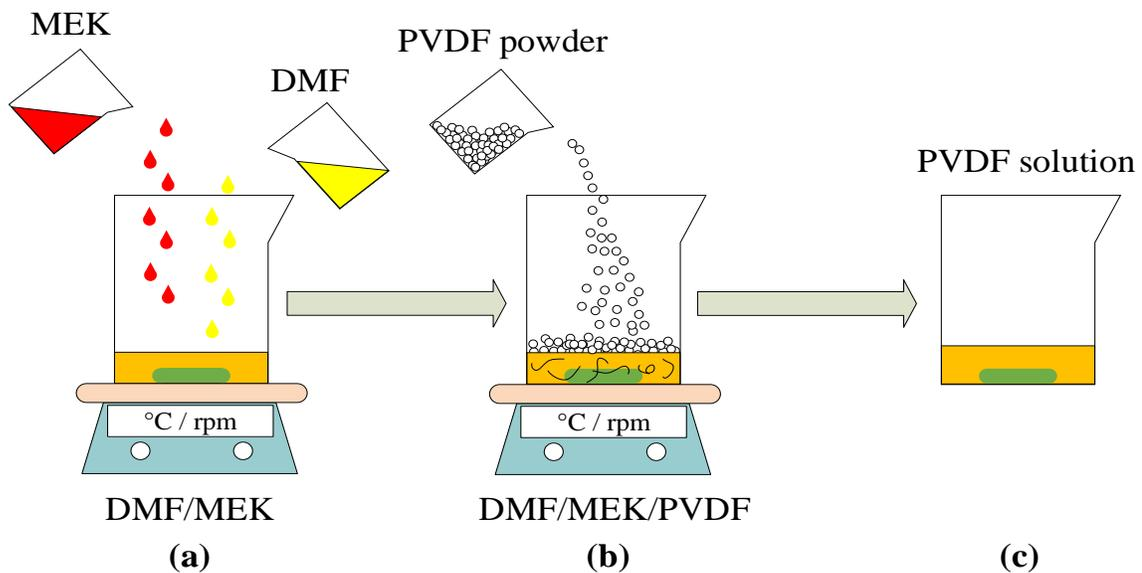
*Figure 19.* Dissolving method for PVDF. a) MEK and DMF are poured into a beaker. The beaker is placed on a hot plate which is set at 70°C. b) Once the solvent's temperature reaches 70°C, PVDF is poured into the beaker and stirred at 300 rpm for 50 min. c) Uniform PVDF solution.
