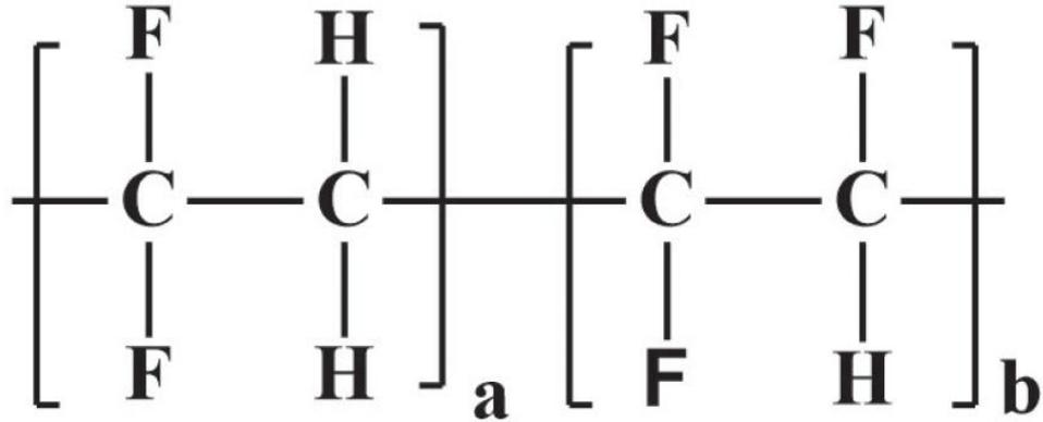
Figure 11. Chemical structure of PVDF-TrFE [15].
