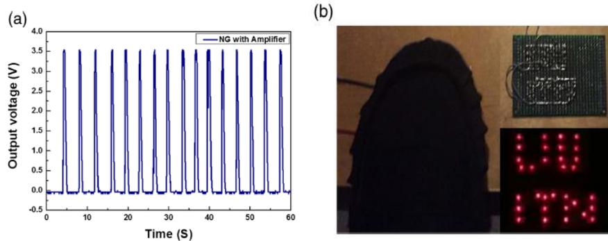
*Figure 13.* a) The average output voltage. b) The energy-harvesting circuits connected to LED display triggered by foot pressing [77].
