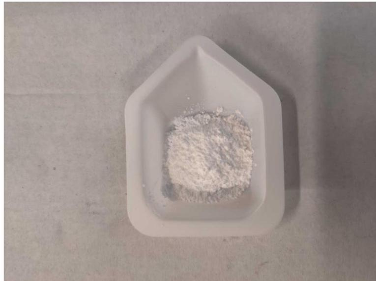
*Figure 15.* Powder PVDF used in our experiments.
