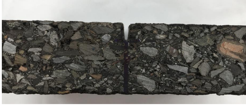
Figure 9. Notched asphalt sample.
