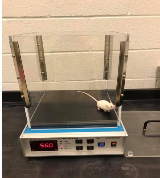
Figure 8. Hot Plate Apparatus. Image of hot plate apparatus with a CD-1 mouse from our research lab. The hot plate has an aluminum flat surface maintains 56-degree Celsius temperature. There is a switch to turn on and a built-in timer.
