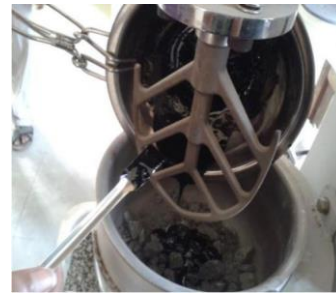
(b) Adding the Blend to the Heated Aggregates
