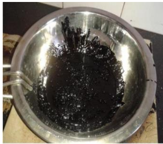
(a) Polypropylene Fiber Mixed with Asphalt Binder
