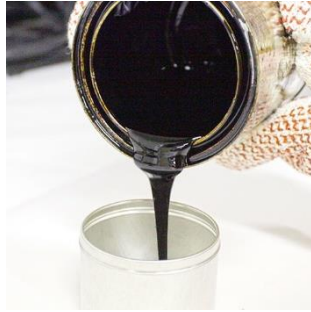
(a) Asphalt binder
