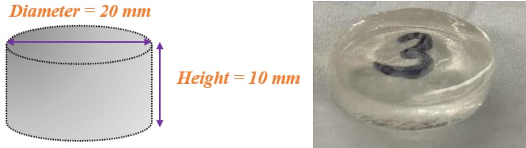
Figure 15. Specimen used for compression
