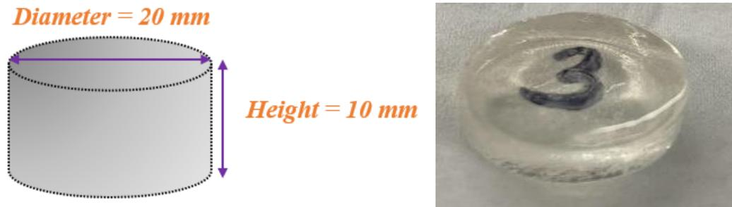
Figure 15. Specimen used for compression
