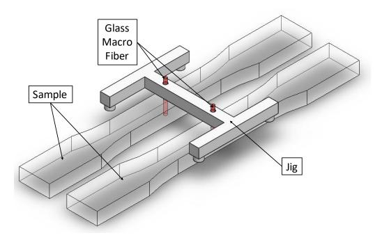
A similar approach was followed to prepare 2-fiber samples. Separate jigs were fabricated and used for each orientation of the two-fiber samples. The jigs were printed on an Ultimaker 2+ with a 0.6 mm nozzle with ABS. After printing it was found that the holes as printed were undersized for the glass fiber so then the holes for the glass fiber were brought to a workable size by using a drill bit to slightly enlarge them to a clearance
