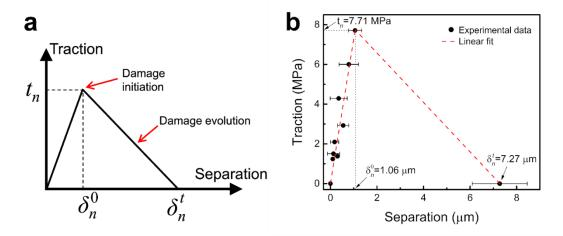
By analyzing our full-field measurements, we can directly extract the three parameters mentioned. By examining the local strain values obtained for the top and bottom of the fiber-matrix interface (**Figure 9a**), damage initiation was found to occur at a global tensile stress of  $\sigma^{\infty}$ =5.35 MPa. This stress can be evaluated at the interface of the fiber and matrix using the classical solution provided by Goodier [27], and later referenced in [11] as:
