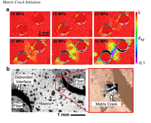
With the previously mentioned observations, the assumption can be made that the coalescence of the shear bands formed between the fibers in multifiber samples (**Figure** 10) is a primary cause for failure within their matrix. The existence of a link or how
