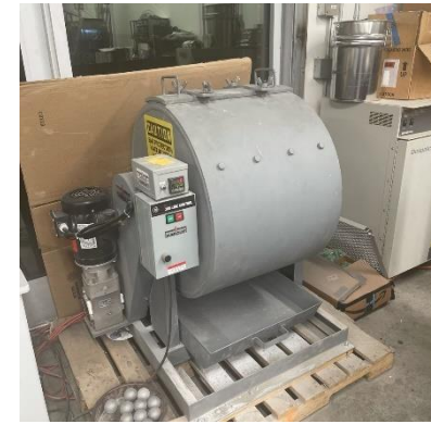
Cantabro Durability Test
