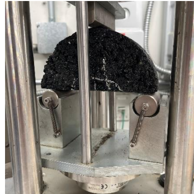
SCB Cracking Test
