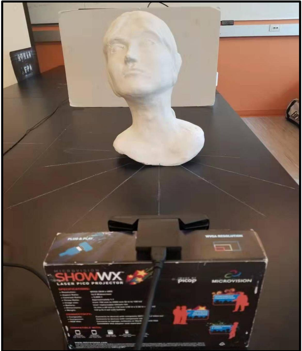
The camera was kept still, while the object was gradually displaced following the marked angle lines underneath covering the entire object from front to back. shown in Fig. 5. The data were then captured and collected using our project-camera calibration system [18]. The stitching algorithm was implemented using MATLAB. Various combinations of tests were carried out to explore the optimal solution.
