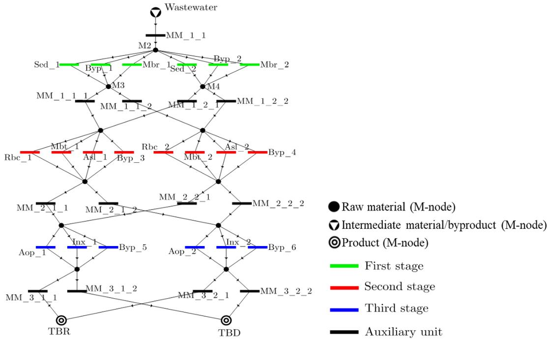
Figure 18. Maximal structure for coffee case study. TBR – To Be Recycles; TBD – To Be Discharged.
