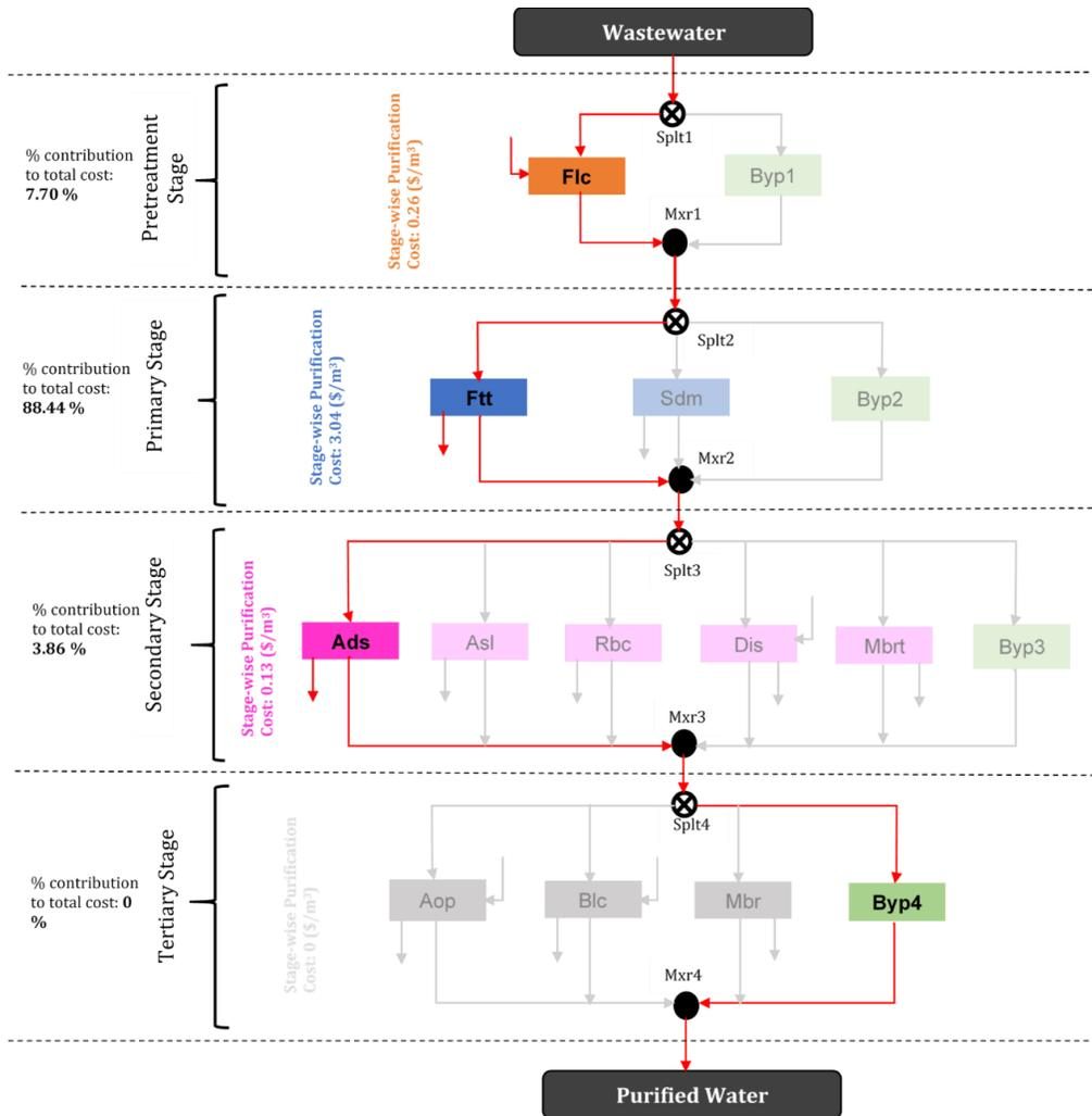
Figure 12. Optimal treatment pathway for pharmaceutical wastewater treatment
