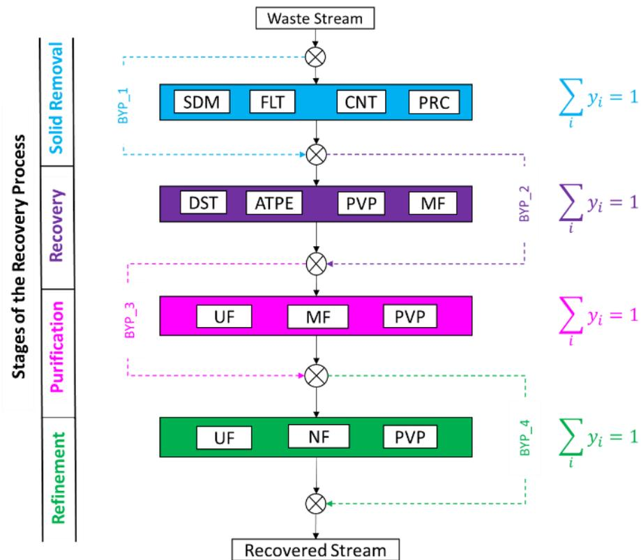
Figure 21. Superstructure for waste solvent recovery showing technologies, streams, and bypasses (SDM – Sedimentation; FLT – Filtration; PRC – Precipitation; CNT – Centrifugation; DST – Distillation; ATPE – Aqueous Two-Phase Extraction; PVP – Pervaporation; MF – Microfiltration; UF – Ultrafiltration; NF – Nanofiltration; BYP\_1,2,3,4 – Bypasses 1,2,3, and 4
