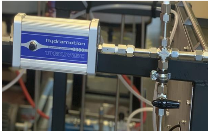
Figure 32. Inline Viscometer for Real Time Viscosity Measurement
