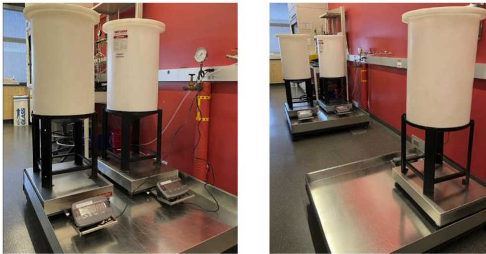
Figure 29. Polyethylene Product Storage Tanks - 30 Gallons Capacity, Measuring Scales and Metal Foundations
