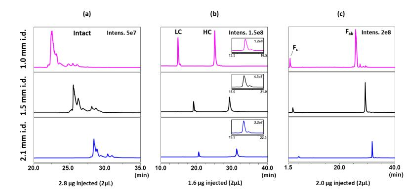
*Note:* The  $1.0 \times 150$  mm (top, pink traces),  $1.5 \times 150$  mm (middle, black traces), and  $2.1 \times 150$  mm (bottom, blue traces) Halo 1000Å Diphenyl 2.7 µm columns showing MS full scan [800–4000 m/z, 3-point moving average smoothing applied] chromatograms. 2.8 µg of intact trastuzumab (a), 1.6 µg reduced and alkylated trastuzumab and inset of light-chain peak (b), and 2 µg of IdES-digested trastuzumab (c) were analyzed on each column.
