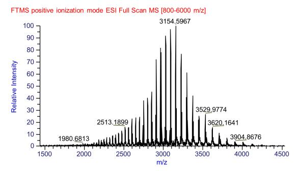
*Note*: Mass Spectra from  $0.040\mu$ L injection of  $0.5\mu$ g/ $\mu$ L (20ng on-column) intact trastuzumab separated on a 1000Å Diphenyl 0.3x150mm  $2.7\mu$ m. The spectrum was obtained by averaging 25 spectra across the peak at 2.46 min. The experiment was performed on an Axcend Focus LC capillary liquid chromatography system coupled to a Thermo Q Exactive HF mass spectrometer.
