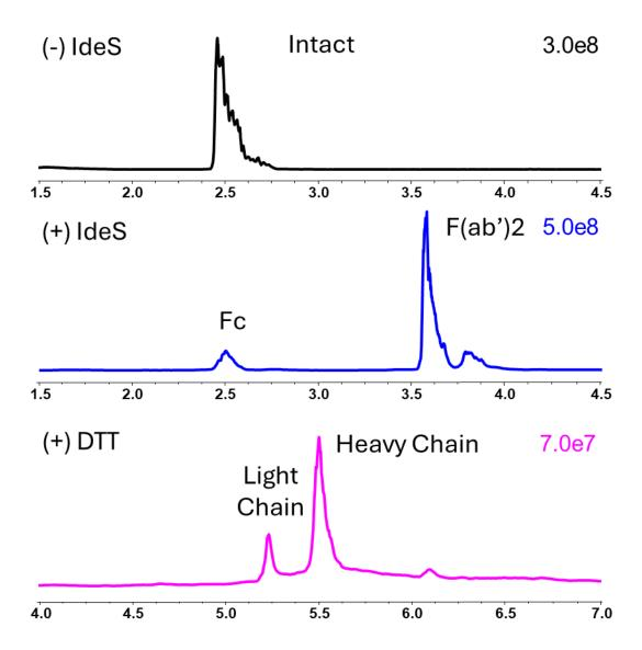
*Note:* Total Ion Current chromatograms from intact and subunit trastuzumab separated on a 1000Å Diphenyl 0.3x150mm 2.7 $\mu$ m column. The experiment was performed on an Axcend Focus LC capillary liquid chromatography system coupled to a Thermo Q Exactive HF mass spectrometer. The capillary LC system was operated at 7  $\mu$ L/min with gradients of 25-52.5%B over 5 min for (+) IdeS, 20-50%B over 7 min for (-) IdeS, and 10-67%B over 10 min for (+) DTT.
