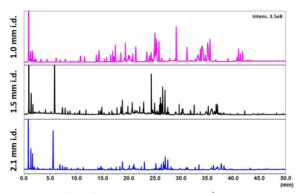
*Note:* Separation of 1  $\mu$ g of trastuzumab digest on ES-C18 160Å 2.7  $\mu$ m 1.0 × 150 mm (top, pink) 1.5 × 150 mm (middle, black) and 2.1 × 150 mm (bottom, blue) columns. Full scan total ion current chromatograms are shown (300-2000 m/z).
