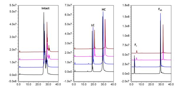
LCMS Replicate Injections of Intact and Subunit mAb on 2.1 and 1.5 mm i.d. Columns
