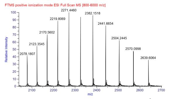
*Note*: Mass Spectra from trastuzumab  $F(ab')^2$  subunit separated on a 1000Å Diphenyl 0.3x150mm 2.7µm. Average of 95 spectra displayed for peak at 4.10 min. The experiment was performed on an Axcend Focus LC capillary liquid chromatography system coupled to a Thermo Q Exactive HF mass spectrometer.
