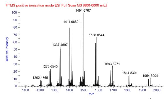
*Note:* Mass Spectra from trastuzumab Fc subunit separated on a 1000Å Diphenyl  $0.3x150mm 2.7\mu m$ . Average of 40 spectra displayed for peak at 2.98 min. The experiment was performed on an Axcend Focus LC capillary liquid chromatography system coupled to a Thermo Q Exactive HF mass spectrometer.
