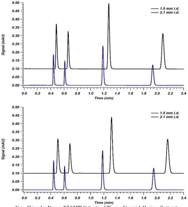
Note: Shimadzu Nexera X2 UHPLC (top) and Thermo Vanquish Horizon (bottom).
