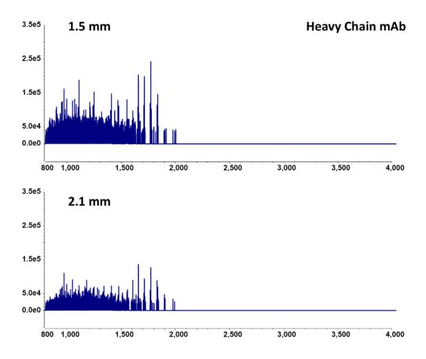
Trastuzumab Fc Mass Spectra From 1.5 and 2.1 mm i.d. Column Experiments
