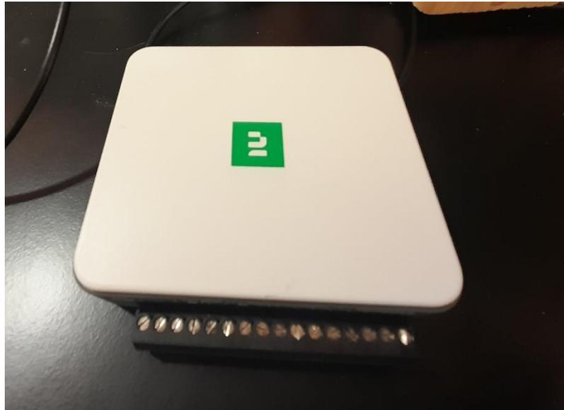
*Figure 26.* National Instrument (NI) USB-6000 multifunction data acquisition (DAQ) device
