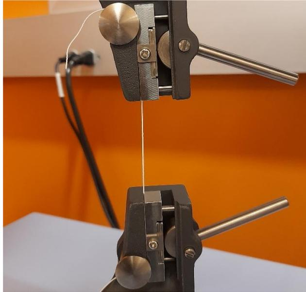
*Figure 24.* Tensile test of an electrospun PVDF-HFP nanofiber yarn using the universal testing System
