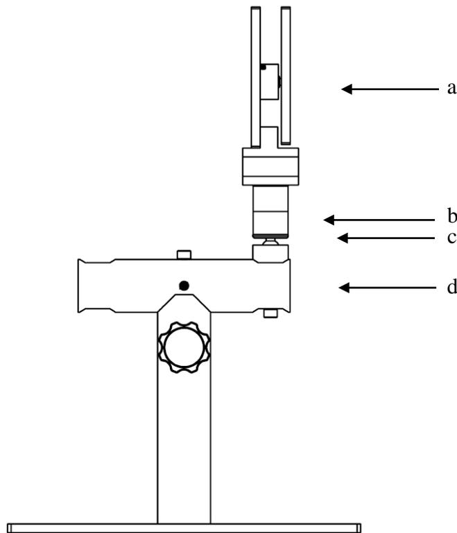
*Figure 15.* A drawing of the device, including (a) the handheld fixture, (b) the adaptor, (c) the ball-and-socket joint, and (d) the adjustable base. The ball-and-socket joint and adaptor were added to this assembly to reduce the possibility of damage to the tri-axial transducer due to eccentric forces.
