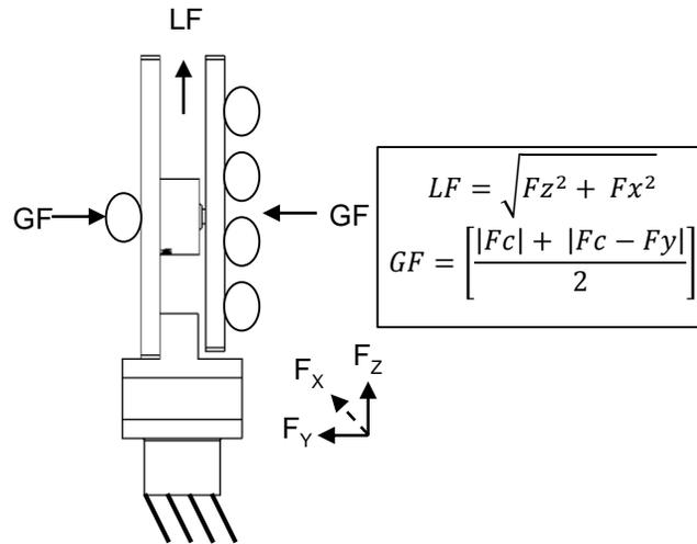
*Figure 1.* Schematic illustration of the handheld portion of the experimental device with a simplified view of the instructed finger placement. The single-axis force sensor measured the compression force,  $F_C$ , while the tri-axial transducer measured  $F_X$ ,  $F_Y$ , and  $F_Z$ . These forces were used in the equations shown to calculate the grip force,  $GF$ , and the load force,  $LF$ .
